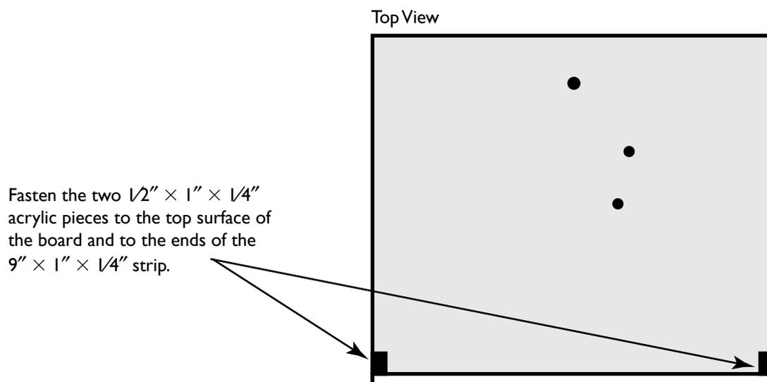
7. Position the two  $4\frac{1}{2}'' \times 1'' \times \frac{1}{4}''$  acrylic strips on the top surface of the board, along the sides. Leave about a  $\frac{1}{16}''$  gap to the  $\frac{1}{2}''$  pieces that you attached in step 6 (see figure below). Fasten the strips into place using the same technique as above.
