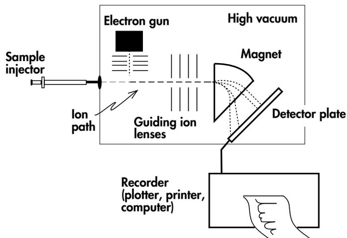
Schematic showing main components of a mass spectrometer.
