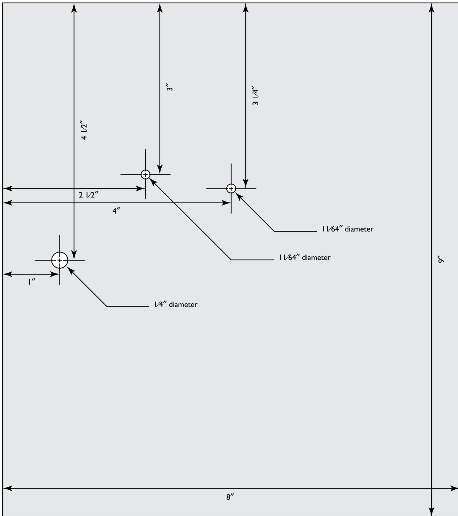
Template for drilling the 9" x 8" acrylic piece of the mass spec demonstration board. (Scale: 1 inch = 1 inch)
