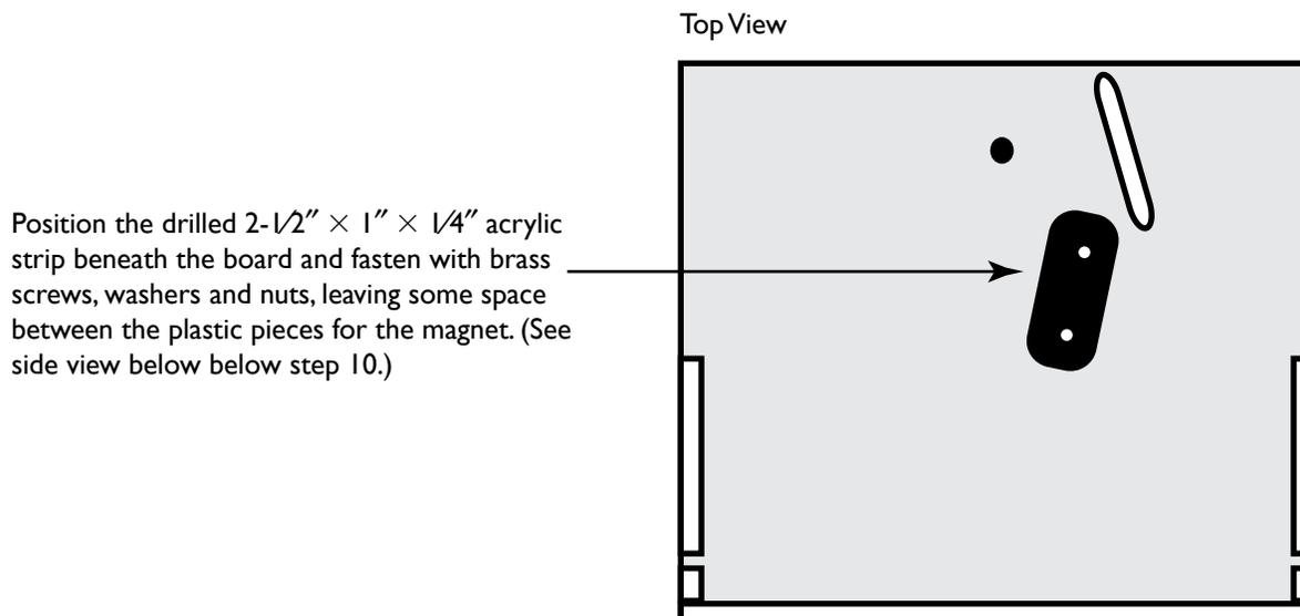
10. Place the alnico magnet between the board and the strip underneath the board. Tighten the nuts to hold the magnet firmly, but allow some motion to adjust its position slightly.
