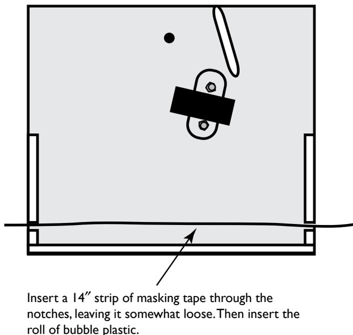
13. Both the slope of the board and the position of the magnet determine the trajectories of the ball bearings down the demo board. Each ball bearing should have its own trajectory, preferably landing as far away from the other bearings as possible. It is easiest to fine tune the trajectories by sliding and rotating the magnet, millimeter by millimeter, about its original position until optimal conditions are reached.
