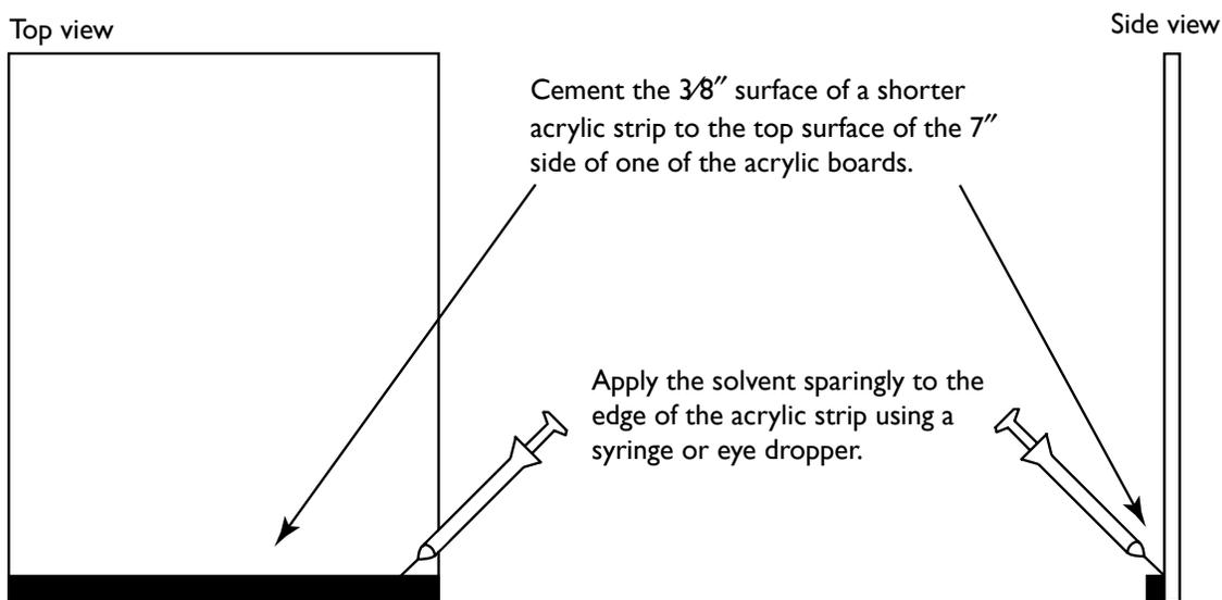
4. Position the two longer acrylic strips along the sides of the 9" × 7" board. Using the same technique as you did in step 3, cement these two strips to the 9" × 7" board and to the edges of the bottom acrylic strip.
