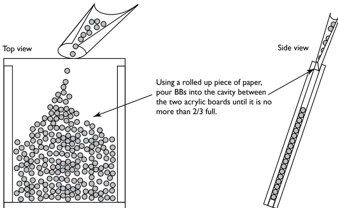
7. To seal the BBs inside the cavity, place the second short acrylic strip between the two acrylic boards. Using a minimum amount of solvent, cement the 3/8" surfaces to the inside surface of each acrylic board.
