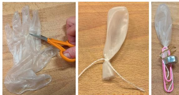
*A finger cut from a lightweight plastic glove can make a diver. The plastic is light so lots of ballast is needed.*
