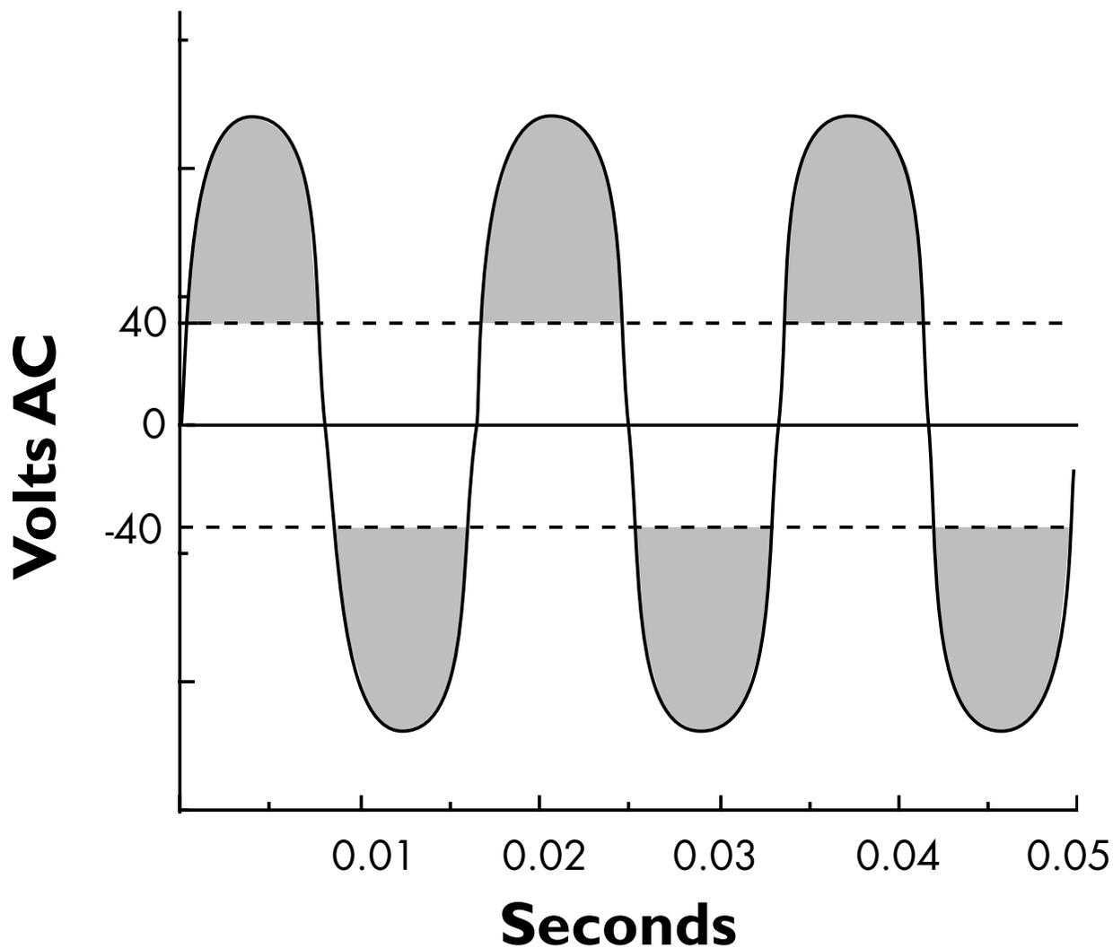
**The neon lamp is on when the voltage is more than 40 volts or less than -40 volts.**
