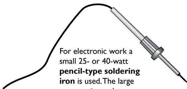
For electronic work a small 25- or 40-watt **pencil-type soldering iron** is used. The large gun-type irons do not have a fine enough tip.
