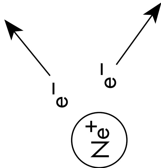
**Step 2. The impact strips off an electron, leaving a neon cation.**
