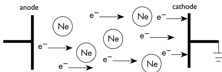
Figure 1. A neon lamp at  $\pm 40\text{V}$ .
